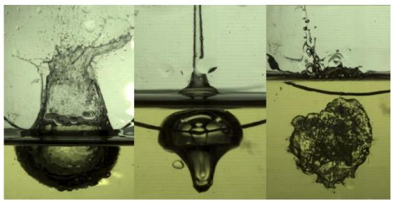
Typical experimental images from my research, where a water droplet exploded in the heated oil (e.g., cavitation) (Kiyama, et al., submitted).
