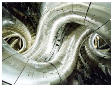
Inside of the LHD vacuum vessel
